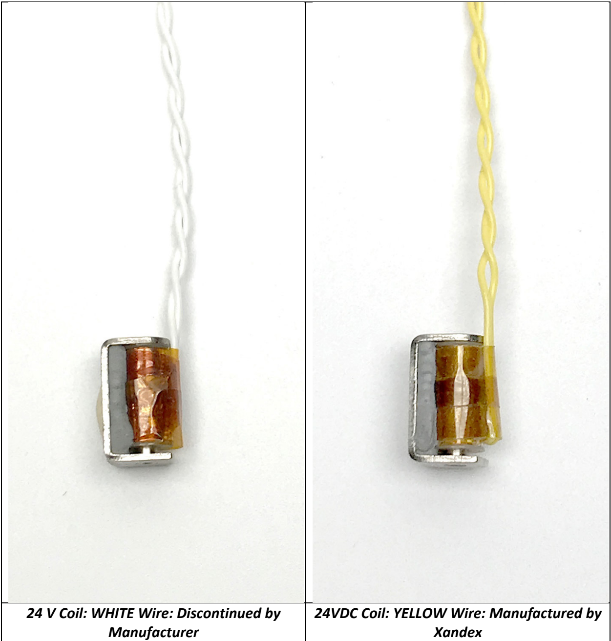
Figure 4. 24VDC Coil wire color changed from white to yellow
